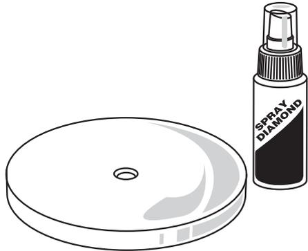
Hold the spray nozzle 3" - 4" from the rotating lap surface and spray a band near the outer edge of the lap surface. About a one second burst is adequate. You will be mostly using the outer 1" - 1-1/2" of the lap surface, so concentrate the diamond there. Cutting action will gradually decrease through use and a short burst of spray will then be needed.
