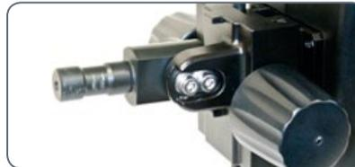
3. Retighten both Allen screws on the connecting pin of the focusing arm. This also locks the tilt.
