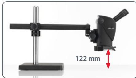
In addition, the focusing arm of the Leica A60 F provides a travel path of 50 mm that is used for focusing on the specimen. This provides you with plenty of freedom to focus on locations with different heights on a printed circuit board, for example.
