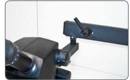
2. Tighten the fastening lever if necessary to protect the stereomicroscope from accidental height adjustment.
