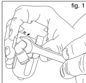
There are 4 screws on each side of the Airtact. Looking at the front of the unit, remove the screw located on the right side, top-rear. Using the same screw, attach the bracket (#044-051) and tighten firmly. Place the filter under the bracket and use the 2 screws (#022-978) supplied with the kit to attach it.
