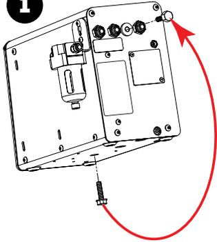
Remove the screw protruding from the bottom of the machine. Insert it with the washer into the rubber grommet located on the back of the machine.
