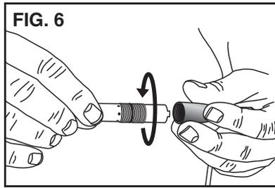
With the handpiece disassembled, clean the parts with a non-residue solvent like denatured alcohol. Make sure the holes in the handpiece body are clear from dirt and debris. DO NOT allow moisture in the air hose. Before reassembly, make sure everything is dry.
