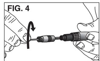
After loosening you can turn the chuck retainer out with your fingertips (FIG. 4). As you pull out the chuck, there will be a spring and piston.
