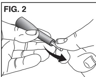
hose back (FIG. 2) into the knob until you see the tip of the brass fitting protrude through the side of the knob. This must be an air-tight fit, so you will have to pull somewhat hard (a few pounds, at least).
