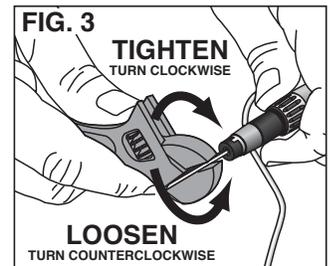
To disassemble the handpiece, use the crescent wrench or pliers to grip the graver (FIG. 3) and turn it counterclockwise to loosen the chuck retainer.
