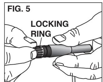
Loosen the locking ring and remove it (FIG. 5).
